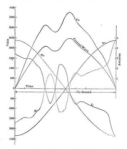
FIG. 47. Diagram showing the e.m.f. waves necessary to send a given current wave through 700 ohms res., 3 henrys inductance, and 20 m.f. capacity.
